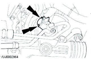
2. CAUTION: Make sure both the retaining bolts are tightened an even number of turns.
