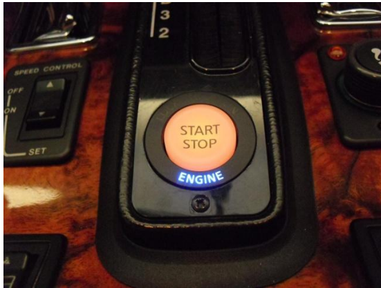
When a door is opened the start button and the blue “engine” sign light up along with the interior lights for 10 seconds
