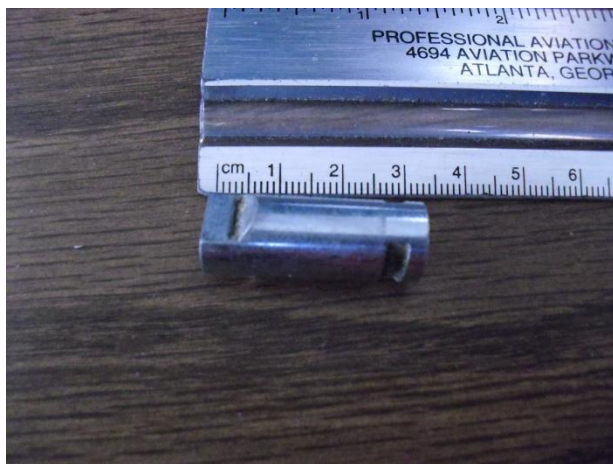
XJS steering wheel locking pin in OEM ignition switch
