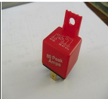
The Bosh type relay K3, K4, K5 & K6
