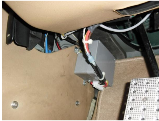
The grey Relay Module on the left kick panel. Notice the white teflon connector strip at the end of the wires
