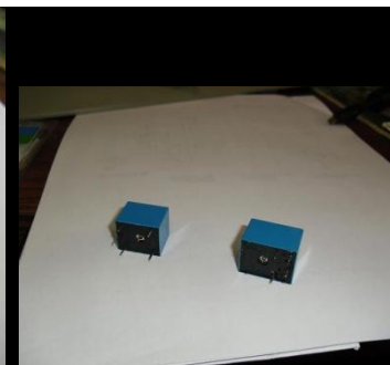
The mini relays in the 12volt ON-OFF latch circuit
