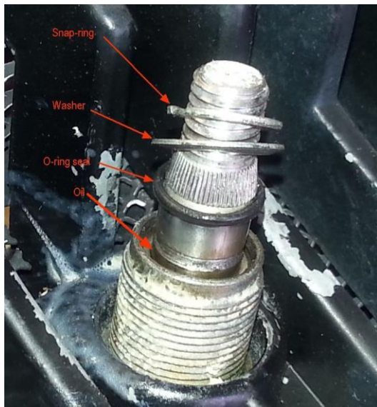
Figure 6 Removing post upper washers & seal
