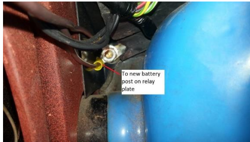
Figure 28 Firewall Power Post
