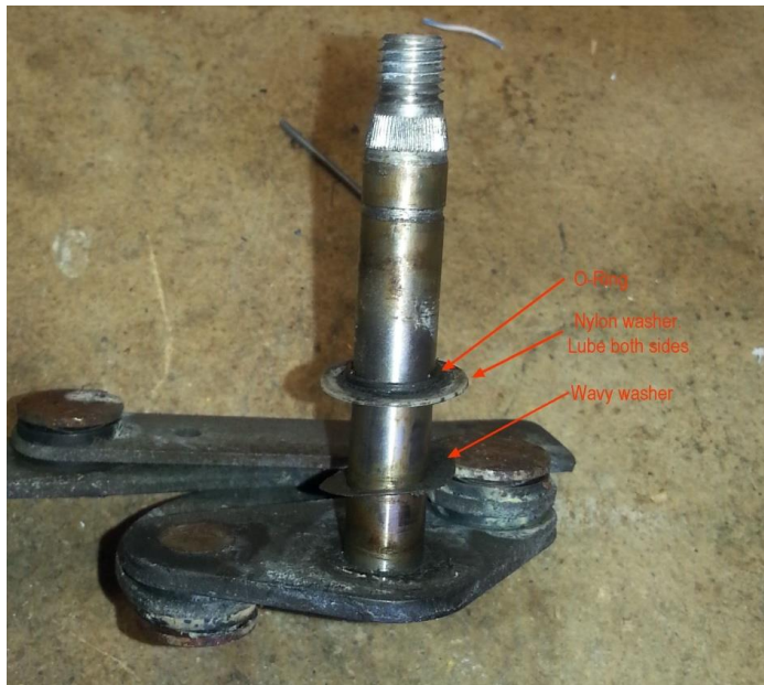
Figure 7 Left arm post & lower washers & seal.
