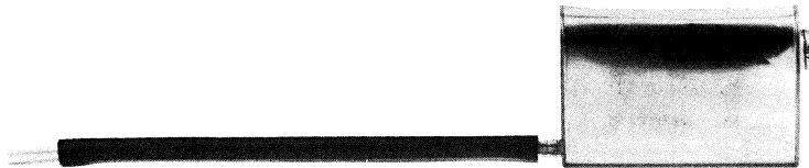
FIGURE 5 - FUEL PERMEATION RESERVOIR TEST - ASSEMBLY STORAGE POSITION
