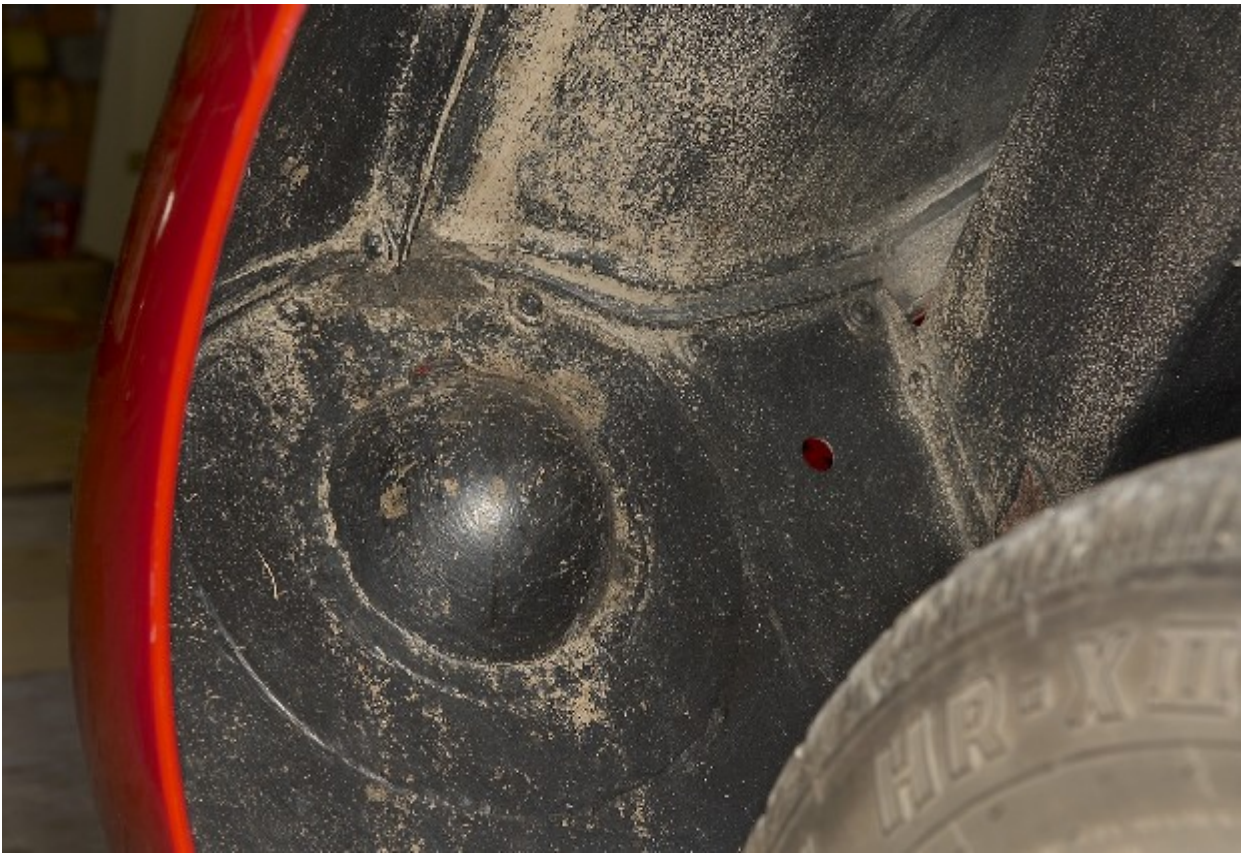
Here's a view of the rear panel that I had to modify. With the headlamp bowl now sitting further back, I had to modify this panel. All I did was cut out the centre area then solder in a cut down part from another set of headlamp bowls.
