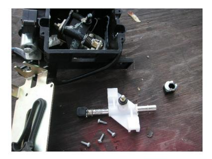
The Welsh aluminum metal slider goes on either way, but check the movement of the oblong lever. Mine was not quite right one way but good the other way. Put grease on the slider and ball ends.
