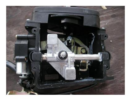
Reattach side cover and replace J-gate using magnetic screwdriver or magnet on stick to start screws. Shifter set in R. Push in cable end one click for R and connect swivel end. Snug up 2 nuts, check movement through all positions. Connect small cable. Check movement. Tighten nuts.
