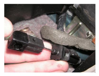
The small cable running forward controls the key locking in the ignition switch, and must be pulled back to release the key. Notice the black plastic oblong lever on the right side. This must swing up all the way to pull the small cable out, otherwise you can't remove the key.
