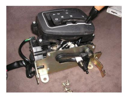
Remove 4 screws on the gold anodized side cover. White plastic slider and shaft with rubber ends lift straight out.
