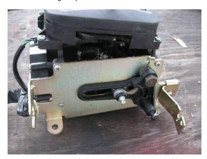
The solenoid on the back of the shifter prevents movement without the brake pedal. The small microswitch on top tells the computer if the shifter is in J-gate mode or regular PRND mode.
