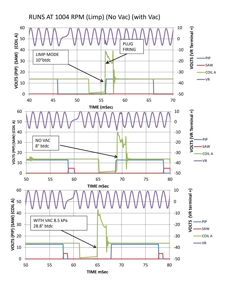
The USB output from the Megajolt was recorded over a range of speeds and manifold vacuum to see how it tracked with the desired advance characteristics. *Quite well as it turned out.*
