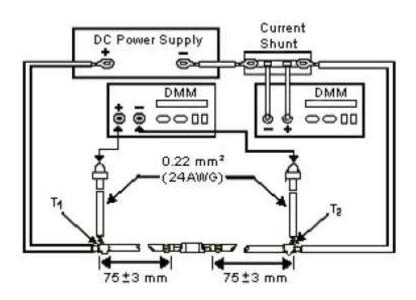
mVD Entire Connection = mVD(T1 - T2) - [mVD Conductor ]
