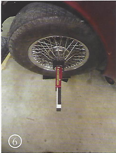
[FIG 7] Castor here is showing 2 degrees positive. The gauge must be centered on the hub.
