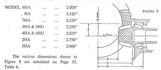
Thus, for a model 3HA pinion marked Minus Two (-2) the distance from the centre of the drive gear to the face of the pinion should be 2.248" (i.e. 2.250"—.002") and for a pinion marked Plus Three (+3) the cone setting distance should be 2.253".
